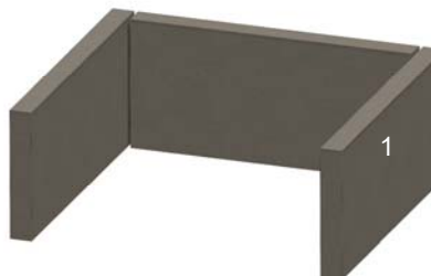
Figure 9. Riser Legs & Cross-Leg
